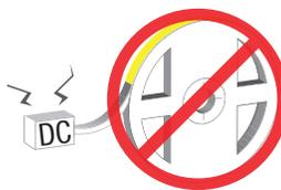
**Do not power while attached to spool or tightly coiled.**
