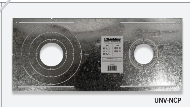
Allows positioning of fixture locations between ceiling joists before sheetrock is installed. Galvanized steel plate has break-out rings for specific fixtures. Use as guide for hole cut-outs.
