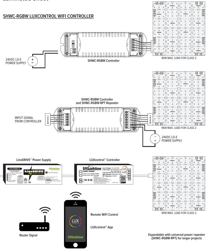
Note: For use with LD-E (non-dimmable) or LD-ED (dimmable) power supply only. Not compatible with LD-MD (magnetic) power supply.
