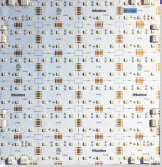
Sheets can be rotated to get cut lines into the best orientation for the application. Align all sheets the same way.
