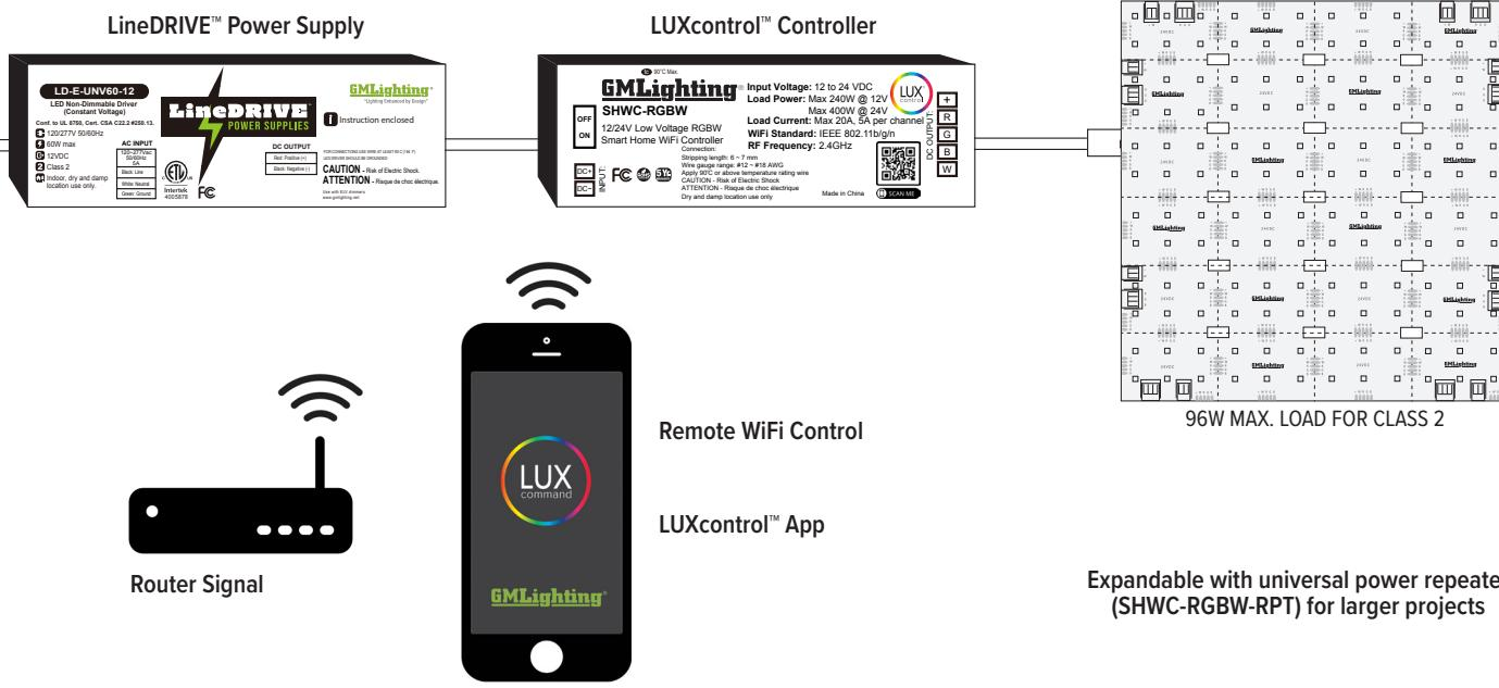
Note: For use with LD-E (non-dimmable) or LD-ED (dimmable) power supply only. Not compatible with LD-MD (magnetic) power supply.
