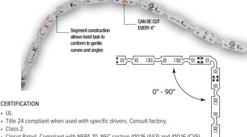
• Closet Rated. Compliant with NFPA 70, NEC section 410.16 (A)(3) and 410.16 (C)(5)
