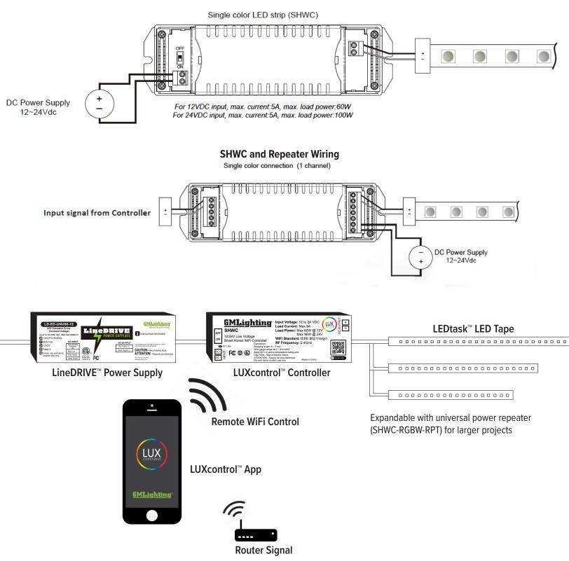
**Note:** For use with LD-E (non-dimmable) or LD-ED (dimmable) power supply only. Not compatible with LD-MD (magnetic) power supply.
